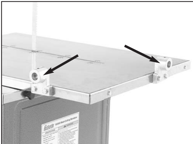
Figure 25. Fence supports to table.
